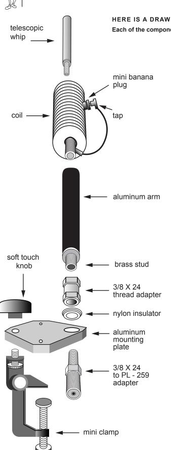
HERE IS A DRAWING OF THE BUDDISTICK. Each of the components is marked for ease of assembly.
